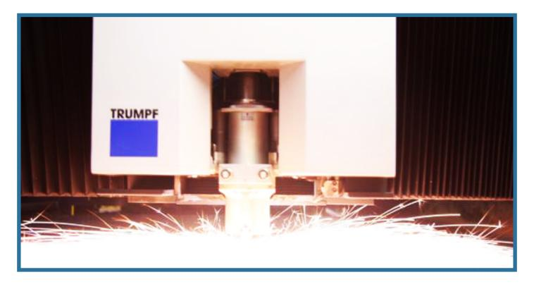
The laser cutting facilities can be applied to various material types – mild steel, stainless steel and aluminium and will provide the undernoted material specific cutting capacity:
