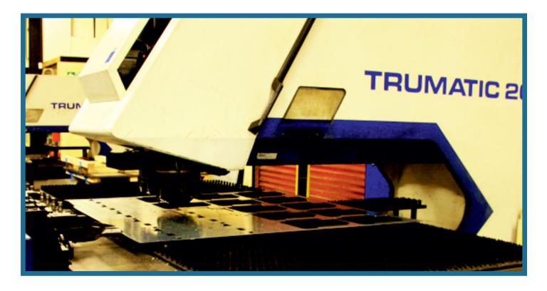
The punching facilities are capable of acceleration rates of up to 1200 strokes per minute and all parts are programmed utilising the in-house CAD system.
